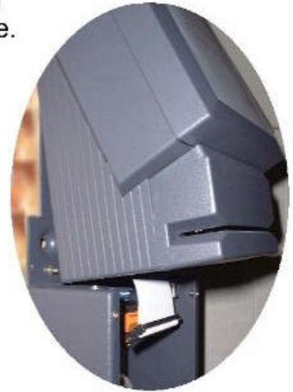
(4) Tilt bottom of TimeClock forward off of lugs and lift off of flange in top of Wall Base.
