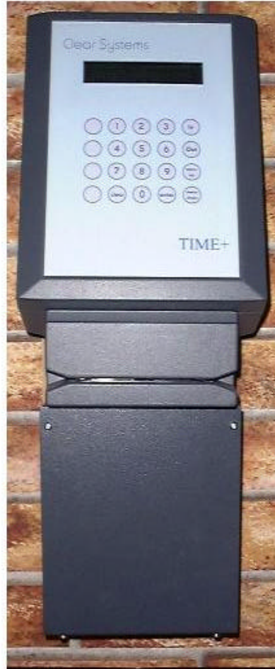
(4) Tilt bottom of TimeClock forward off of lugs and lift off of flange in top of Wall Base.
